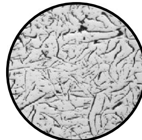
Effect of MI Inoculant In Gray Iron X 100
